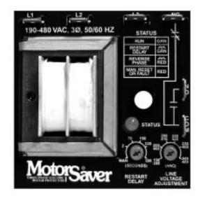
**Model 202** is an auto-ranging voltage monitor designed to protect three-phase motors regardless of size. It is used on 190-480 VAC, 50 to 60 Hz motors to prevent damage caused by single phasing, low voltage, high voltage, phase reversal, or voltage unbalance.
